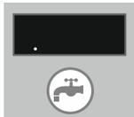
When the DHW mode is selected the display will show the actual temperature in the DHW accumulation tank. The boiler will always give priority to DHW production over central heating until the selected DHW temperature is reached.
