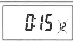
The optimum start control must be adjusted to match the building energy characteristics. Use the **Λ** and **V** keys to selected the required pre-heat period. The table below suggests typical settings. If the building fails to reach temperature on time, increase the setting by 15 minute steps each day until the correct setting is found. If the building reaches temperature ahead of time, decrease the setting by 15 minute steps each day until the correct setting is found.
