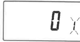
Use **Λ** and **V** keys to enable or disable the function (1=enabled, 0=disabled).
