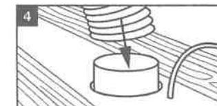
Place flexible ducting over the spigot of the fan.
