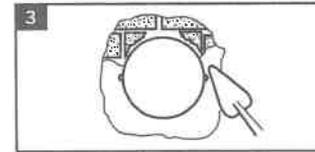
Fill in any gaps with mortar or foam and make good internal and external walls. Make sure that ducting remains circular and screw holes are horizontal.
