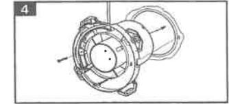
Using No 8 screws, secure fan body to ducting first making sure back draught shutter is fitted, if required, and electrical cable passes through as appropriate. Wire fan (See wiring details).
