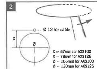
Cut an opening through the ceiling for the fan and electrical cable.
