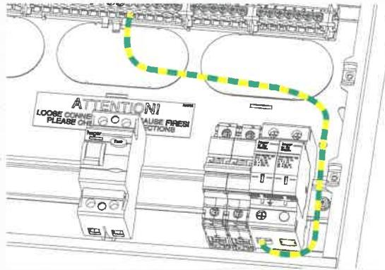
Feed the 6mm earth cable around the side of the main switch as shown and terminate in the earth bar. Torque to 3.6Nm.
