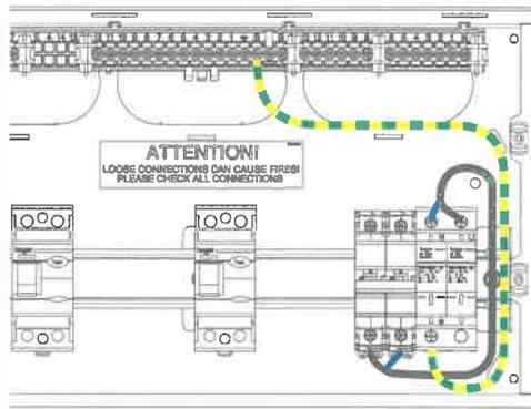
Make sure all cables are secure and torque back to 3.6Nm.
