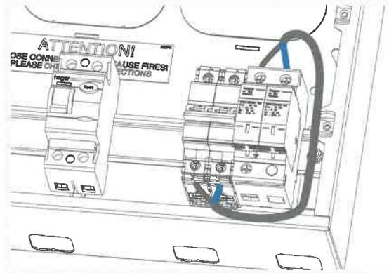
Loosen the L&N screws on the main switch and terminate the spade terminals in the Bi connect.
