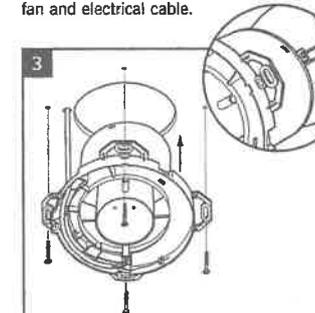
Secure to ceiling using suitable screws first making sure backdraught shutters are removed but shutter spider is left in position. Wire fan (See wiring details).
