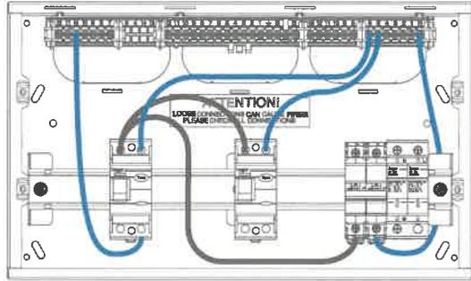
Move the main switch over 2 modules and clip the SPD cable set to the DIN rail.
