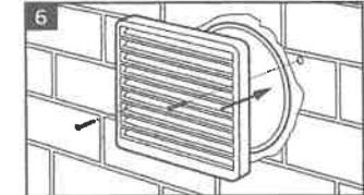
Screw the protective wall grille over the external duct opening.
