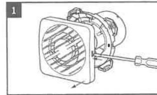
Remove one piece Internal Grille using screwdriver. Push in to free catch then twist to remove grille.
