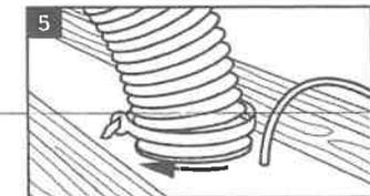
Fit ducting to spigot using ties supplied, making sure impeller rotates freely. Maximum duct length to comply with Building Regulations:
