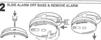
WITH THE SCREWDRIVER STILL INSERTED, PUSH THE LOWER HALF OF THE ALARM AWAY FROM THE SCREWDRIVER, IN THE DIRECTION OF THE ARROW ON THE COVER
