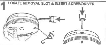
LOCATE THE ARROW ON THE FRONT FACE OF THE ALARM THE SLOT IS LOCATED DIRECTLY ABOVE THE ARROW INSERT A FLAT-BLADED SCREWDRIVER HORIZONTALLY APPROX. 1cm INTO THE CENTRE OF THE REMOVAL SLOT
