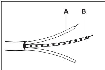
1. Connect the green and yellow (earth) wire to the terminal which is marked with the letter 'E', or the earth symbol  $\oplus$ , or coloured green and yellow.
