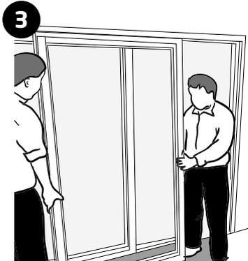
3 Lift the bottom of the door out at an angle and store safely to one side.
