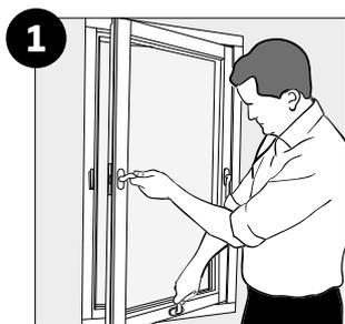
**1** Open the window into the side hung cleaning position (using the side handle on the "opening" side and the bottom handle)
