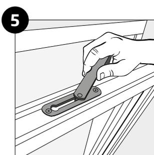
5 Disengage the stay on the top rail of the sash, by sliding the sash to the hinge side of the window.
