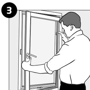
**3** Release the sash from the bottom hinge side corner in the frame
