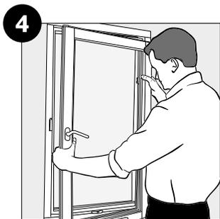
4 Tilt the sash inwards by approximately 30° then lift it up and away from the ball fitting located at the bottom of the 'hinged' side.
