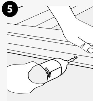
**5** Pre-drill and countersink holes then fix, with one screw 100mm from each end and spaced no more than 500mm apart in between, checking units are straight and level
