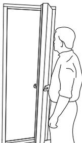
Open the door to approximately 90° or more so that the door blade clears the head of the frame.
