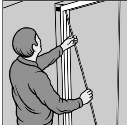
Frame jambs must be square and plumb in both directions and the diagonals should be identical.
