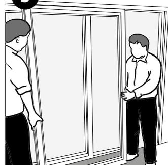
Lift the bottom of the door out at an angle and store safely to one side
