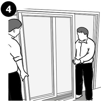
4 To re-install the door carefully replace the door leaf into the frame positioning the top of the door and bringing the bottom of the door in-line with the rollers.
