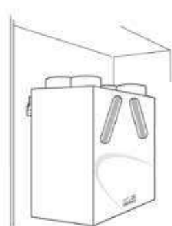
Typical cupboard installation of MRXBOX(AB)-ECO2
