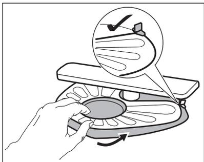
7. Reassemble the filters (B) and (C).
