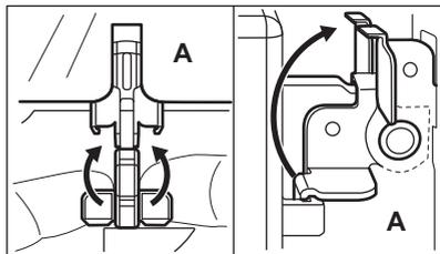
**Step 3** Close the oven door to the first opening position (approximately 45° angle). Hold the door with one hand on each side and pull it away from the oven at an upwards angle. Put the door with the outer side down on a soft cloth on a stable surface.
