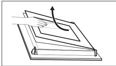
**Step 9** Install the smaller panel first, then the larger and the door. Make sure that the glasses are inserted in the correct position otherwise the surface of the door may overheat.
